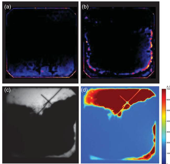
Figure 6.2 ILIT and PL Images of the Group A Cell, (a) ILIT before, (b) ILIT after (c) PL after (d) PL (color scale) after PID Stressing at 60 °C/0% RH, -600 V, 96 h.
