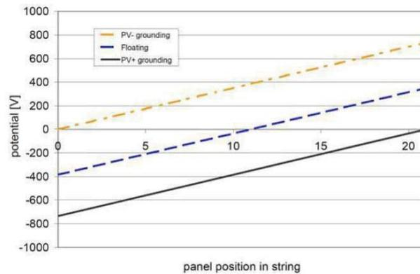
Figure 2.9 Potential Distribution for P-Type Modules in Strings Based on Type of Grounding [28].
