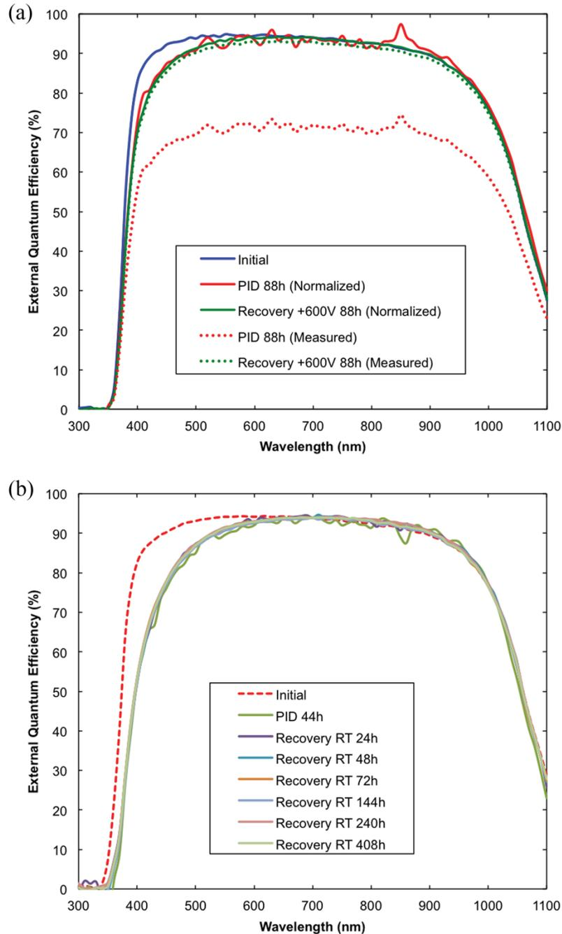
Figure 3.8 (a) QE of Coupon Used in Figure 3.3, QE of Fresh/Initial, PID-Stressed and Recovered Cells (PID Stress at 60 °C/-600 V/88 h; PID Recovery at 60 °C/+600 V/88 h), (b) Normalized QE of Figure 3.6 (a), QE of Fresh/Initial, PID-Stressed and Recovered Cells (PID Stress at 85 °C/-600 V/44 h; PID Recovery at RT/No Bias/408 h).
