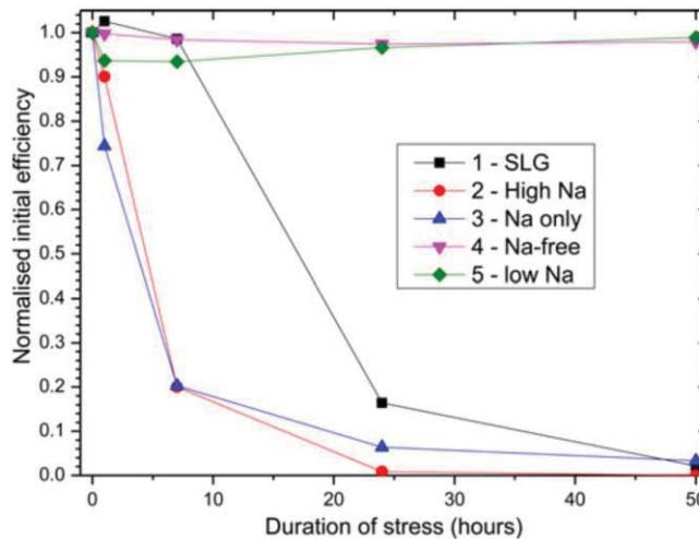
Figure 2.38 PID Susceptibility Depending on the Type of Glass Including Soda-Lime Glass (SLG) Used in the CIGS Modules [88].
