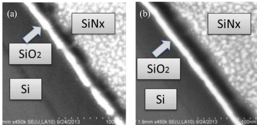
Figure 2.33 SEM Image of a Solar Cell Cross Section of (a) an Ion Implanted Cell and (b) a Modified  $\text{POCl}_3$  Sample, Which has a Diffusion-Furnace-Grown  $\text{SiO}_2$  after Phosphosilicate Glass (PSG) Removal [63].
