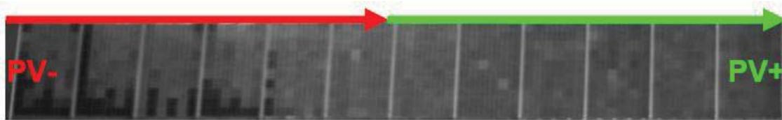
Figure 2.11 EL Image of a Floating Potential String. PID is Stronger in Higher Negative Potential Portions [28].
