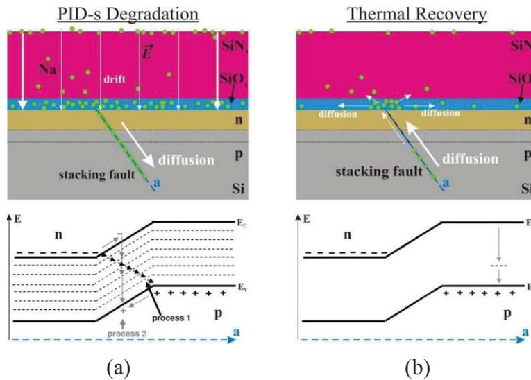
Figure 2.29 Band Diagram Showing (a) Proposed PID Mechanism and (b) PID Recovery Mechanism [48].
