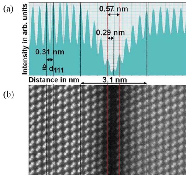
Figure 2.26 (a) Brightness (intensity) and Dimensions of a PID-Affected Stacking Fault; (b) The Corresponding High-Angle Annular Dark Field (HAADF) TEM Image Shows Atomic Structure of the PID-Affected Stacking Fault [35].
