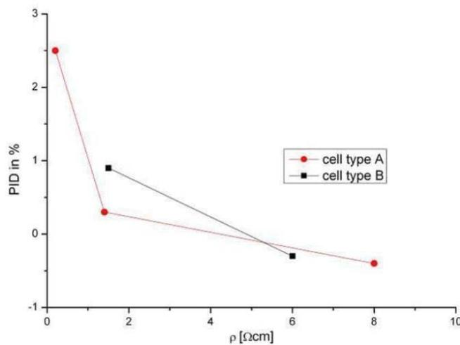
Figure 2.18 PID Susceptibility as a Function of Base Resistivity [28].
