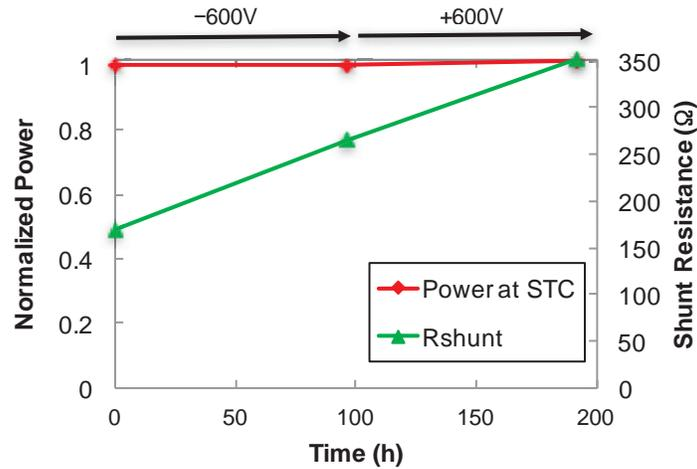
Figure 2.36 PID Test Results of ASU SPL HIT Cell.
