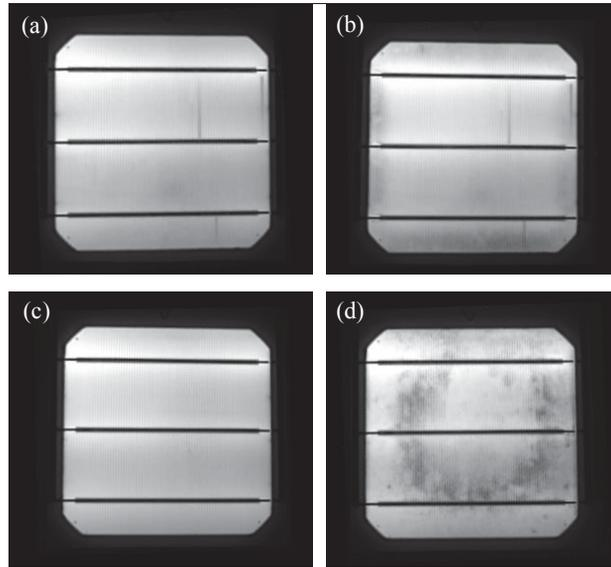
Figure 7.3 EL Image before/after PID-s: (a) Coupon A Initial, (b) Coupon A after PID-s, (c) Reference Coupon Initial, (d) Reference Coupon after PID-s. PID Stress Applied at 60 °C/0% RH (with Aluminum Tape Front Covered), -600 V, 96 h
