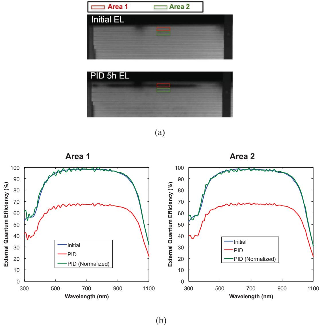
Figure 4.8 EL Image before/after PID and QE in 2 Areas. M2 Cell was used.
