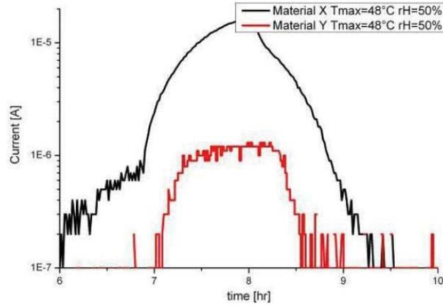
Figure 2.13 Leakage Current of Two Modules Having Different Encapsulant Material but Same Environmental Condition [28].
