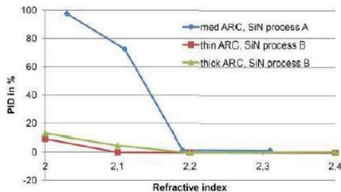
Figure 2.20 PID Susceptibility as a Function of RI, Thickness, and Deposition Process [28].
