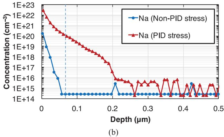
Figure 5.10 SIMS Profiles for Cells Fabricated from Group F and D. PID Stressing at 60 °C/0% RH, -600 V, 96 h (a) Solar Cell with  $\sim 70 \Omega / \text{sq}$  Emitter Sheet Resistance. (b) Solar Cell with  $\sim 60 \Omega / \text{sq}$  Emitter Sheet Resistance.
