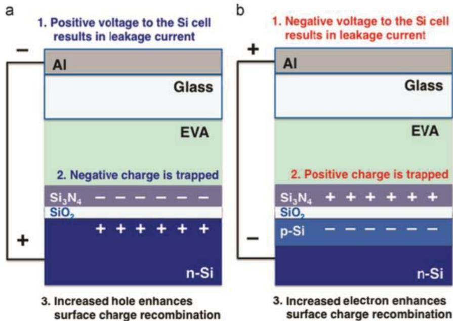
Figure 2.37 Schematic Diagram Shows the Proposed Mechanism of PID-p in N-Type Si PV Modules. (a) N-Type IBC Cell Reported in [27]. (b) N-Type Front Junction Cell [87].
