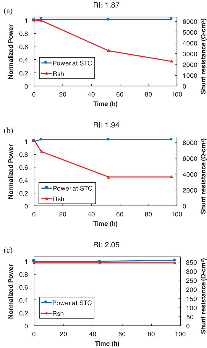
Figure 5.3  $P_{max}$  and  $R_{sh}$  Progression in PID test (60 °C/85% RH, -600 V, 96 h) Cells with Different Refractive Indices. They were encapsulated as One-Cell Coupons with a PV Laminator (a) Group A: RI 1.87  $\text{SiN}_x$  ARC, (b) Group B: RI 1.94  $\text{SiN}_x$  ARC, (c) Group C: RI 2.05  $\text{SiN}_x$  ARC.
