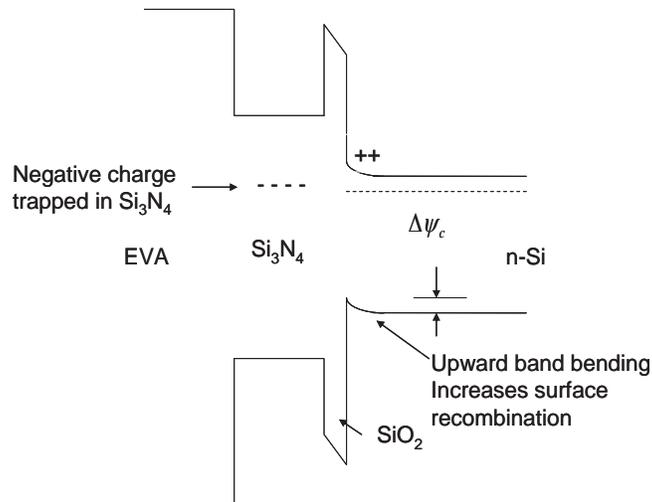
Figure 2.7 Band Structure Showing Polarization [27].
