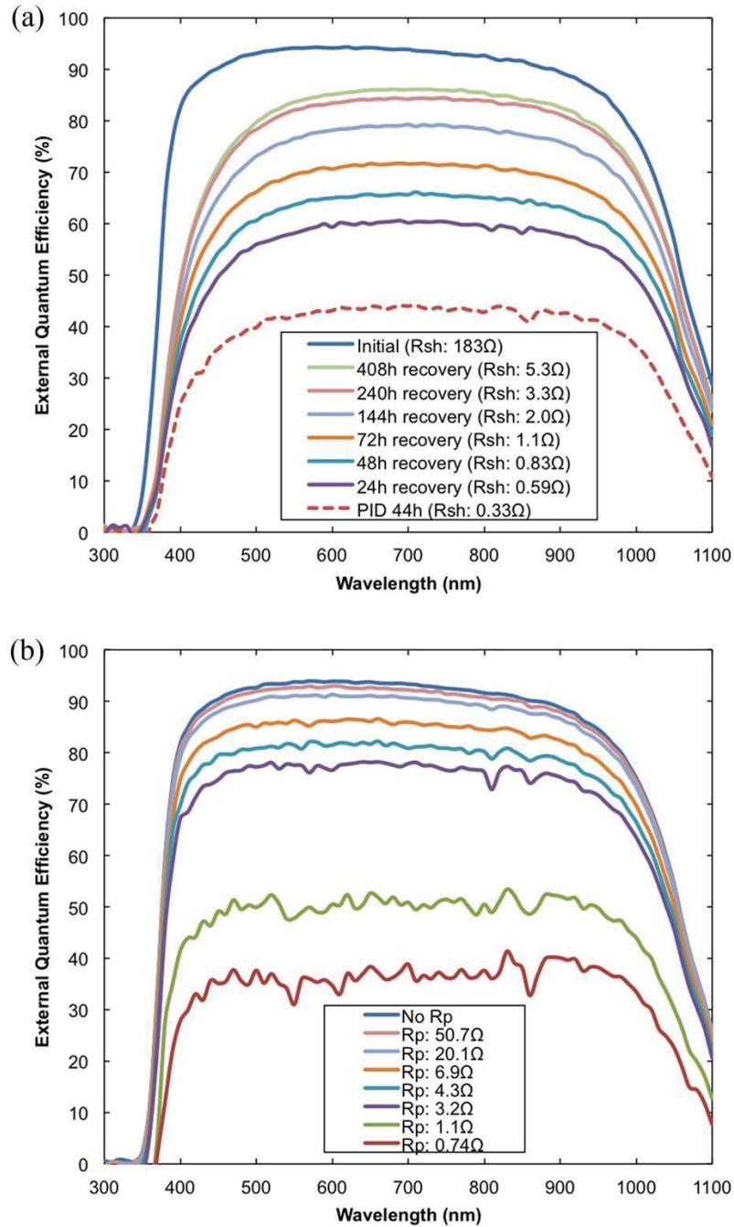
Figure 3.6 (a) QE Curves of Same Test Coupon as Shown in Figure 3.3, (b) QE Curves of a Fresh Cell Coupon Connected with Various Parallel Resistors ( $R_p$ ).
