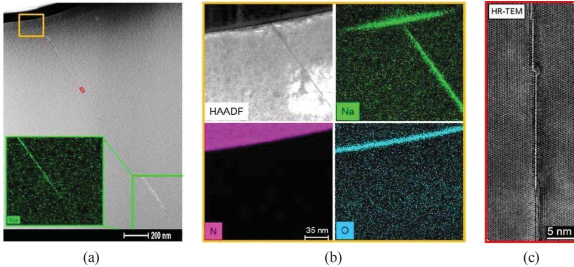
Figure 2.25 (a) TEM Image Showing the Stacking Fault of a PID-Stressed Cell, (b) EDX Intensity Maps Show Sodium Accumulation in a  $\text{SiN}_x/\text{Si}$  Interface and Stacking Fault Area, (c) High-Resolution TEM (HRTEM) Images of the Stacking Fault [42].
