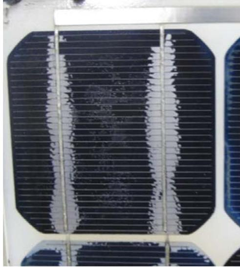
Figure 1.8 PV Module Showing Front-Side Delamination [12]
