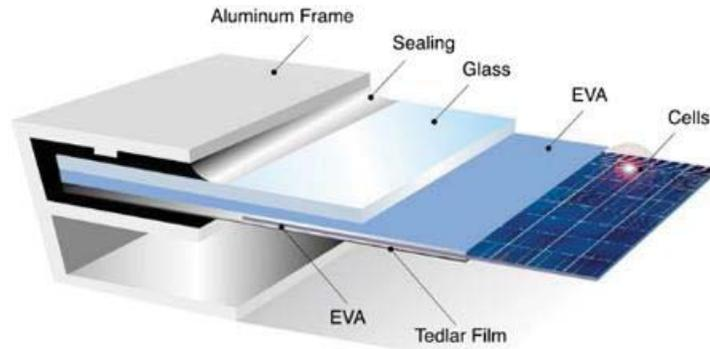
Figure 2.1 Common Crystalline Silicon PV Module Structure.
