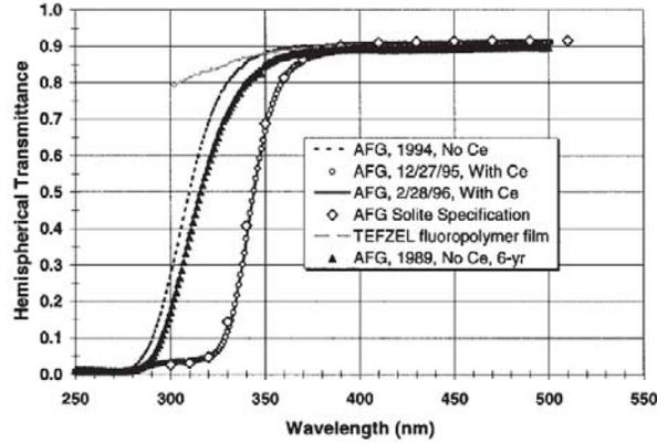
Figure 1.7 Transmittance of Module Superstrate Materials Including Glass Samples with and without Ce Additive [11].
