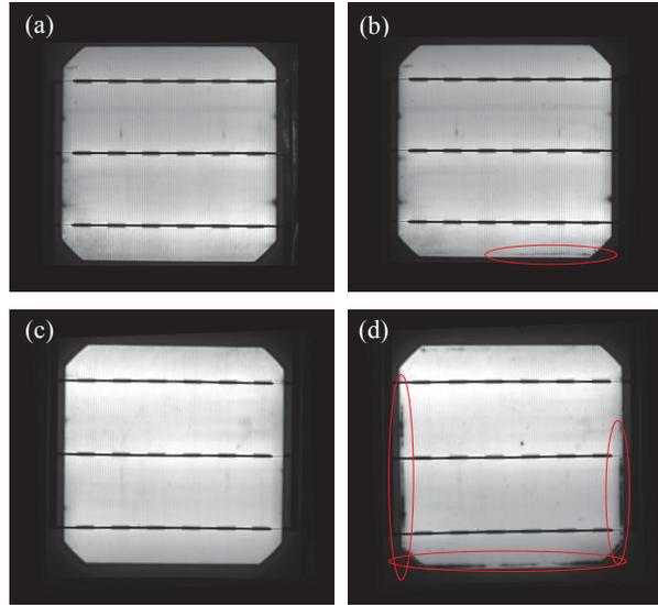
Figure 7.6 EL Image before/after PID-s: (a) Coupon C Initial, (b) Coupon C after PID-s, (c) Reference Coupon Initial, (d) Reference Coupon after PID-s.
