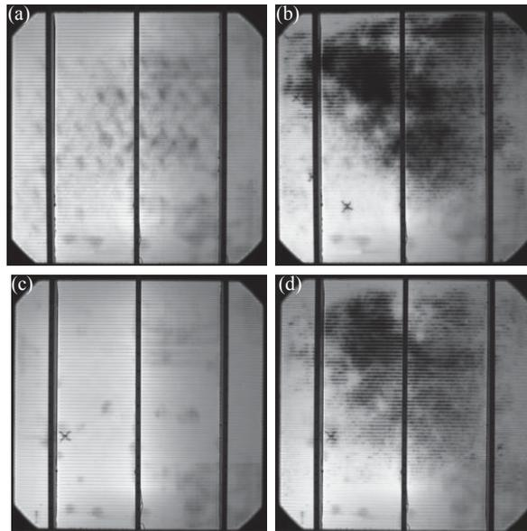
Figure 5.6 EL Images of Different Emitter Sheet Resistance Cells from SPL Pilot Line before/after PID Stress ( $60 \text{ }^\circ\text{C}/0\% \text{ RH}$ ,  $-600 \text{ V}$ ,  $23 \text{ h}$ ). (a) before PID of  $R_{\text{sheet}}: 80 \Omega/\text{sq}$  Cell (Group H), (b) after PID of  $R_{\text{sheet}}: 80 \Omega/\text{sq}$  Cell (Group H), (c) before PID of  $R_{\text{sheet}}: 70 \Omega/\text{sq}$  Cell (Group F), (d) after PID of  $R_{\text{sheet}}: 70 \Omega/\text{sq}$  Cell (Group F)
