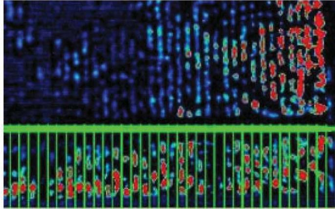
Figure 2.17 Dark Lock-In Thermography (DLIT) Image Showing PID Shunts. Red Areas Represent Shunts [34].
