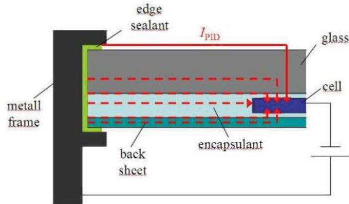
Figure 2.12 Various Leakage Current Pathways from the Metal Frame to the Encapsulated Cell [30].
