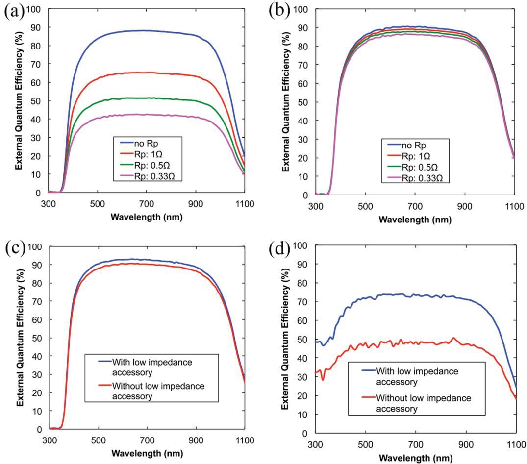
Figure 3.7 Measured QE Curves of a Fresh Cell Coupon ((a) and (b)), PID Cell Coupon (c) and Shunted Cell (d): (a) without Low Impedance Accessory, (b) with Low Impedance Accessory (Three 1- $\Omega$  Resistors were Incrementally Connected in Parallel to the One-Cell Coupon Leads Shown in (a) and (b)). (c) Effect of Low Impedance Accessory on PID-Affected One-Cell Coupon, (d) Effect of Low Impedance Accessory on Heavily Shunted Cell.
