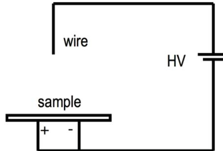
Figure 2.32 Corona Discharge Method for PID Testing [34].
