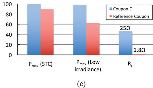
Figure 7.7 I-V Results before/after PID: (a) Coupon C, (b) Reference Coupon, (c) Several Important I-V Parameters Regarding PID.
