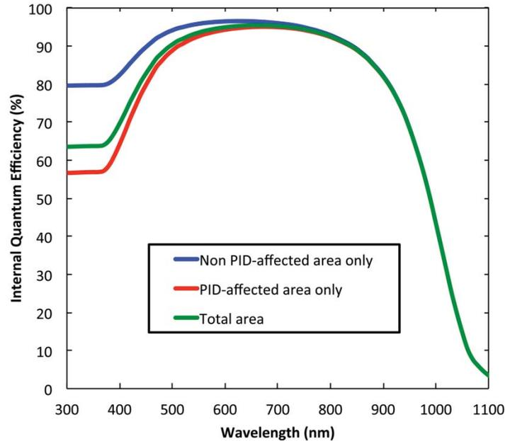
Figure 4.2 Calculated QE to Simulate PID-Affected Cell. Blue Curve is based on Homogeneous Non-PID-Affected Area, Red Curve is based on Homogeneous PID-Affected Area, and Green Curve is based on a Combination of 70% PID-Affected Area and 30% Non-PID-Affected Area.
