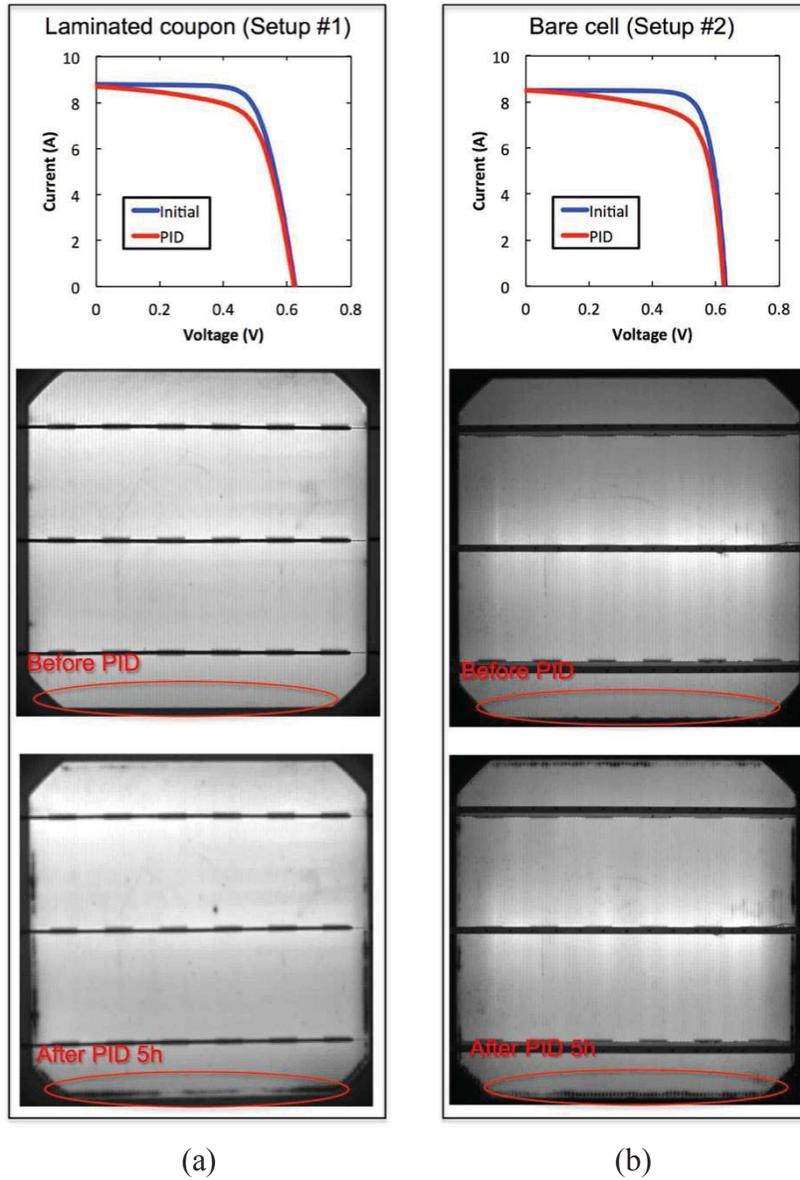
Figure 4.7 Comparison PID Test between (a) Laminated Coupon Method (Setup 1) vs. (b) Bare Cell Method (Setup 2). M2 Cells were used in Both Methods.
