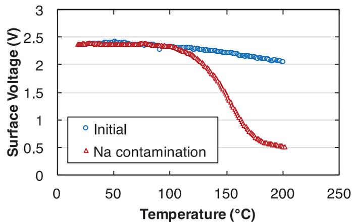
Figure 5.5 Sodium Ion Drift Characteristics of SiN<sub>x</sub> Film (RI: 1.87) Used in This Study for Initial Surface and Intentional Sodium Contamination Surface.
