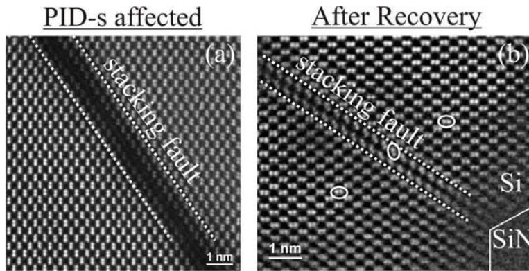
Figure 2.28 HAADF STEM Images, (a) before Thermal Recovery (after PID) and (b) after Thermal Recovery [48].
