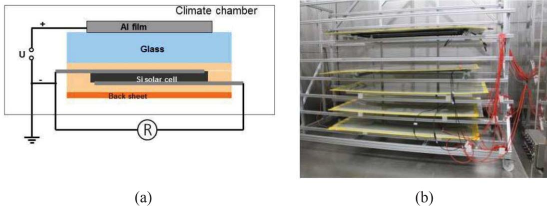
Figure 2.31 Schematic Drawing of (a) the Metal Foil Method and (b) a Photograph [58].
