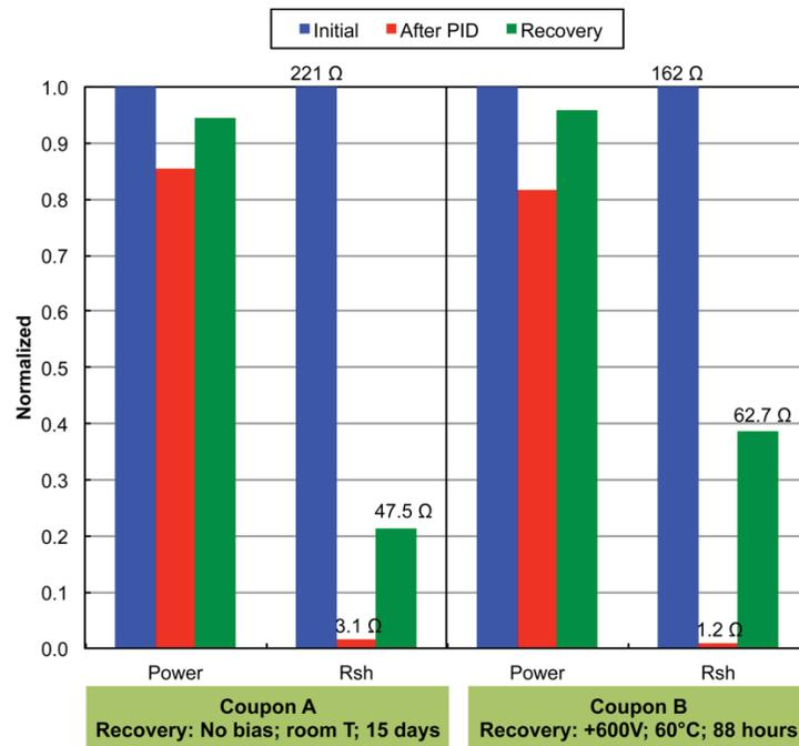
Figure 3.3 Normalized Power and Shunt Resistance. Both Coupons Have the Same PID Conditions ( $60 \text{ }^\circ\text{C}$ ,  $-600 \text{ V}$ , 88 h) but Different Recovery Methods. Coupon A: 15-Day Room Temperature Storage with No Bias, Coupon B:  $+600 \text{ V @ } 60 \text{ }^\circ\text{C}$ , 88 h.
