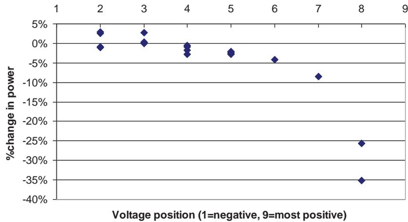
Figure 2.6 Module Power Degradation Distribution due to Polarization in a Series of Connected Strings Installed in an Outdoor Field [27].
