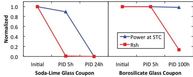
Figure 3.9 PID (60 °C/85% RH, -600 V) Progress of Soda-Lime Glass Coupon and Borosilicate Glass Coupon
