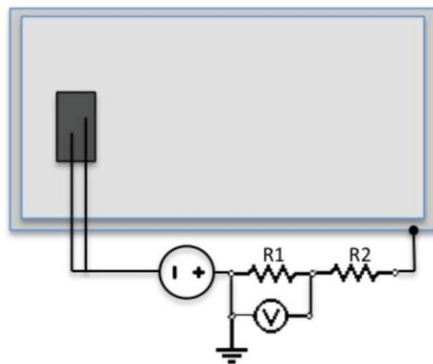
Figure 2.30 A Schematic Showing a PID Setup for the Chamber Method [33].
