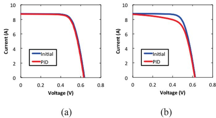
Normalized I-V Parameters after PID
