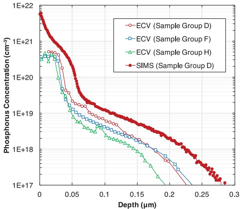
Figure 5.9 ECV and SIMS Profiles for Different Solar Cell Emitters.
