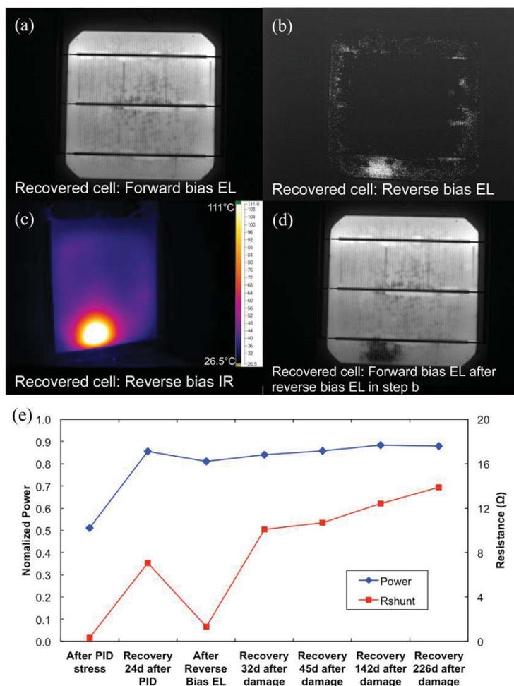
Figure 3.4 EL and IR Images of 24-day RT Stored PID-Stressed (85 °C, 44 h) Cell. (a) Forward-Bias EL, (b) Reverse-Bias EL, (c) Reverse-Biased IR Image, (d) Forward-Bias EL after Cell Damaged by Reverse Bias in Step b. (e) The Recovery Method Applied for These Results is the Room Temperature Storage with No Voltage Application. The Reverse Bias Imposed during EL Decreased the Shunt Resistance. Initial  $R_{sh}$  was 183  $\Omega$ .
