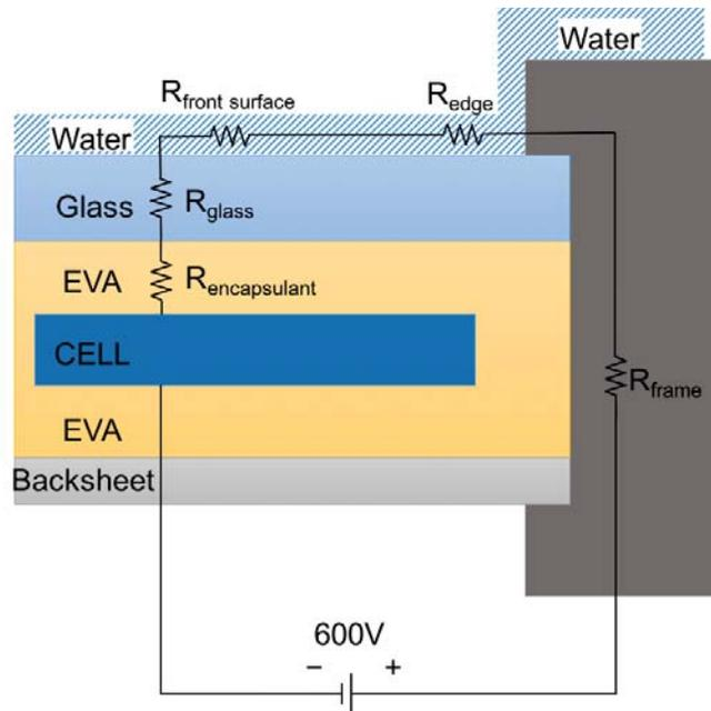
Figure 7.5 Cross-section of Typical PV Module that shows the Resistance of PV Module Materials Affecting PID-s-Susceptibility.
