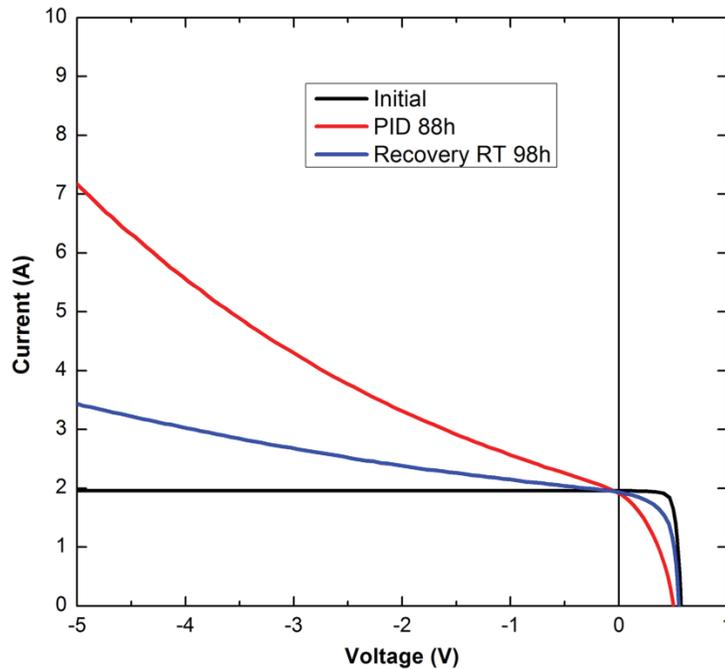
Figure 3.5 I–V Characteristics of PID-Stressed and Recovered Cell at Low Irradiance (240 W/m<sup>2</sup>) (PID 60 °C/–600 V/88 h; PID Recovery at Room Temperature/No Bias/98 h).
