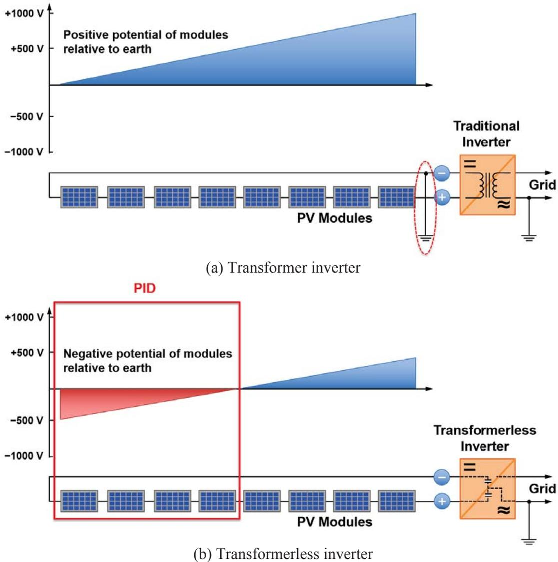
Figure 2.10 Comparison of Transformer Inverter with Transformerless Inverter in a PV System.
