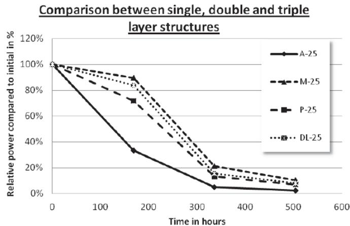
Figure 2.22 PID Degradation from Various ARC Layer Structures. A: Single Layer, DL: Double Layer, and M, P: Triple Layer [37].
