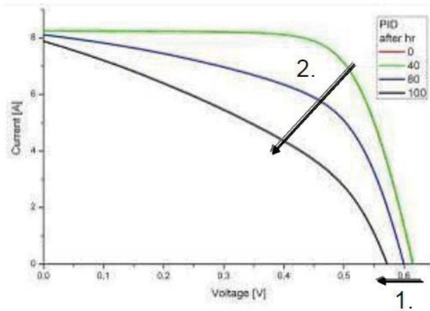
Figure 2.15 Common PID I–V Curves: (1) Shows a  $V_{oc}$  Decrease and (2) Shows an FF Decrease [28].
