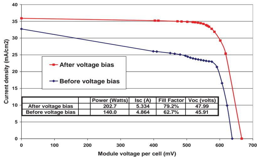
Figure 2.8 Recovery from Polarization by Applying Opposite Potential to The Cells of Degraded Module [27].
