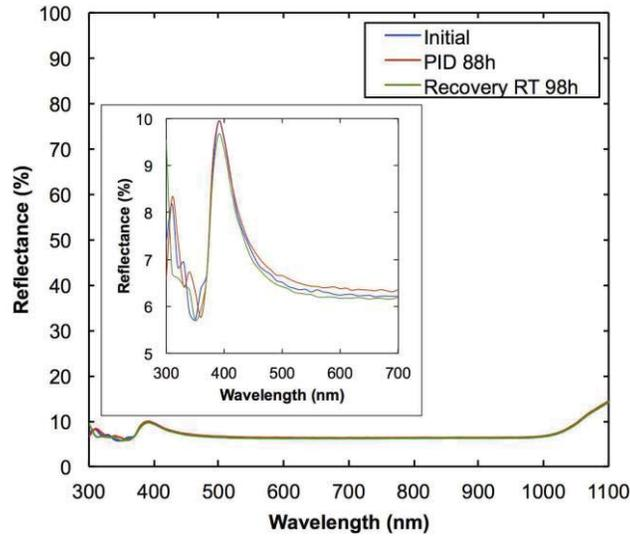
Figure 4.5 Reflectance of a Laminated One-Cell (M1; setup 1) Coupon at Various Stages of Investigation: PID 88 h at 60 °C/0% RH, -600 V, Recovery at Room Temperature (RT). Zoomed-In Plot of Reflectance is shown in a Small Square in Figure 4.5.
