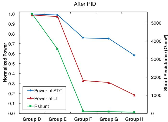
Figure 5.8 PID-Susceptibility with Different Emitter Cells. Values are Post-PID Stress (60 °C, 23 h).
