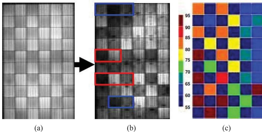
Figure 2.19 PID Results of a Module Containing Cells with Various Emitter Sheet Resistance, EL Imaging (a) before PID and (b) after PID, (c) Emitter Sheet Resistance of Each Cells [34].
