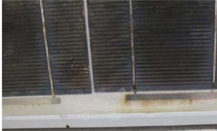
Figure 2.3 Electrochemical Corrosion of Solar Cell after 2000 h in Damp Heat with +600 V Applied to the Cell with Respect to the Module Frame [19].
