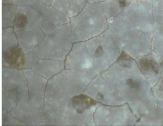
Figure 7.8 Optical Microscope Image (10x) Showing Cracks of the Hydrophobic Layer Sprayed around the One-Cell Coupon Edges.
