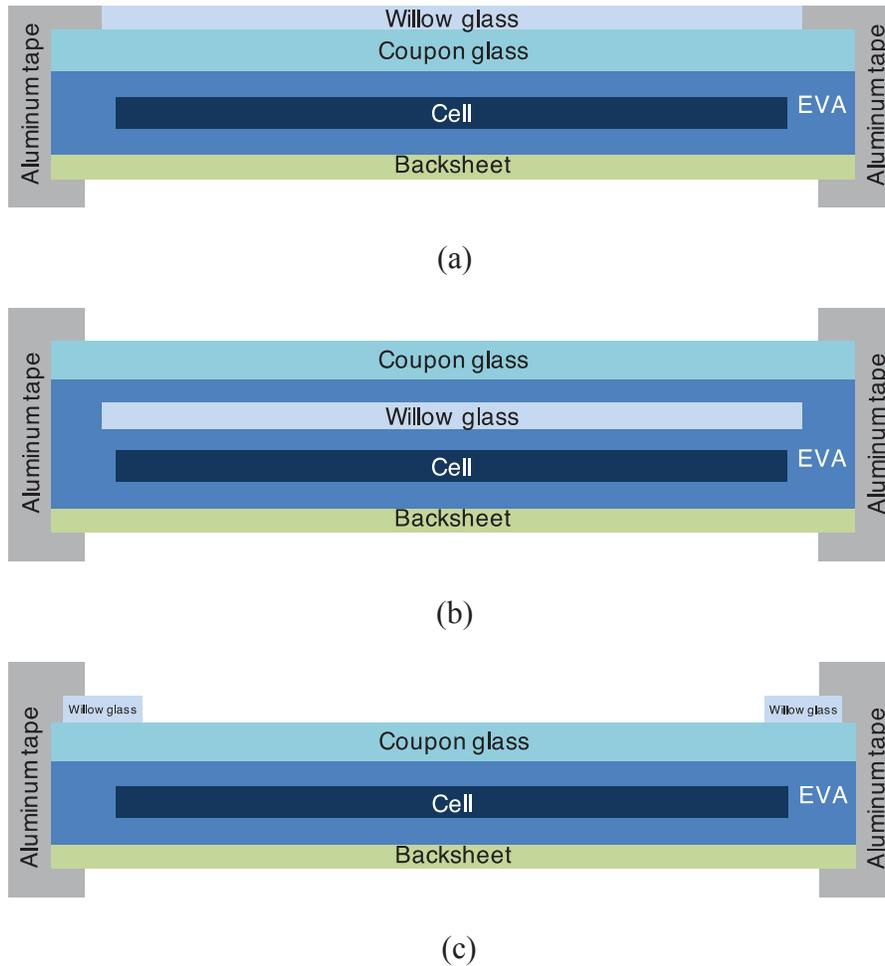
Figure 7.2 Side Views of Coupon with Willow Glass: (a) Coupon A, (b) Coupon B, (c) Coupon C.
