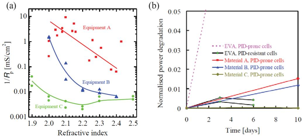
Figure 2.21 (a) Measured Shunt Conductance ( $1/R_p$ ) as a Function of  $\text{SiN}_x$  RI with Different Equipment. (b) Measured Normalized  $P_{\max}$  Degradation from Various PID Modified Modules [36].
