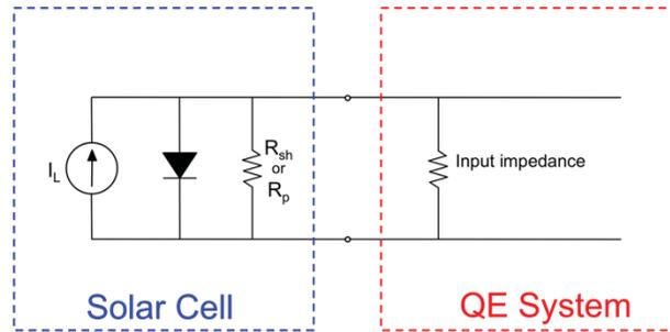
Figure 3.1 Basic Circuit Diagram of a Solar Cell Indicating Shunt ( $R_{sh}$  or  $R_p$ ) and Input Impedance of QE System
