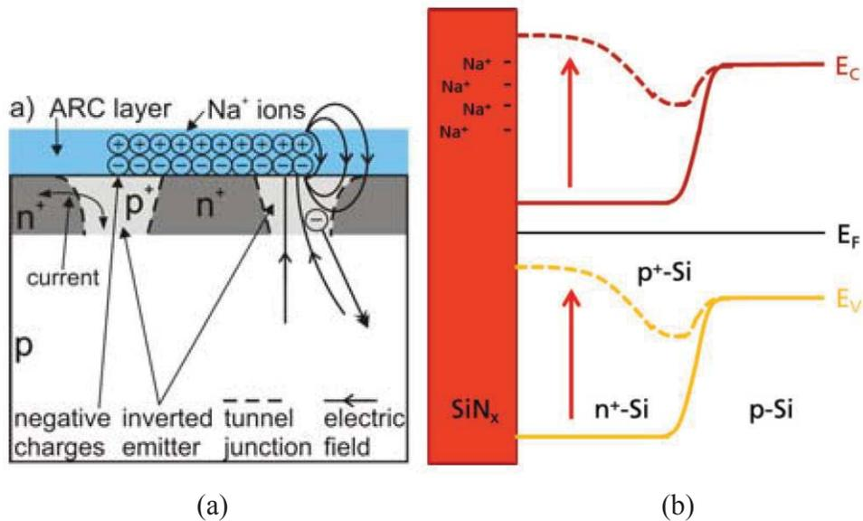
Figure 2.24 (a) Proposed Emitter Inversion Model [40]; (b) Energy Band Diagram Showing Surface-Charge-Induced Band Bending, before PID (Solid) and after PID (Dashed) [39].
