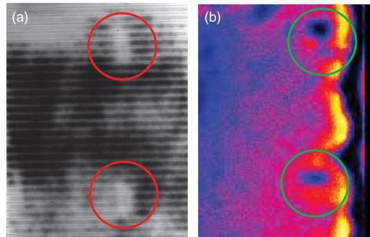
Figure 6.3 Circles in the Images Indicate No PID-Affected Area where 4PP Measured. (a) Enlarged EL Image Shown in Figure 6.1 (b), (b) Enlarged ILIT Images Shown in Figure 6.2 (b), Scale was adjusted to Clearly Show the Effect of 4PP Measurements.
