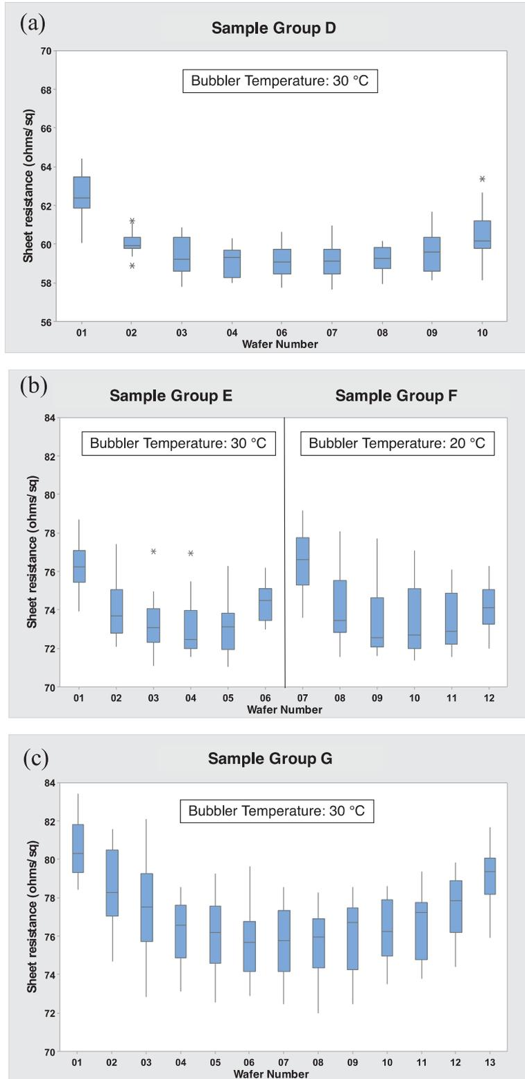
Figure 5.7 Emitter Sheet Resistance Distribution. (a) SPL Standard Diffusion Recipe, (b) Sample Group E and F, (c) Sample Group G.
