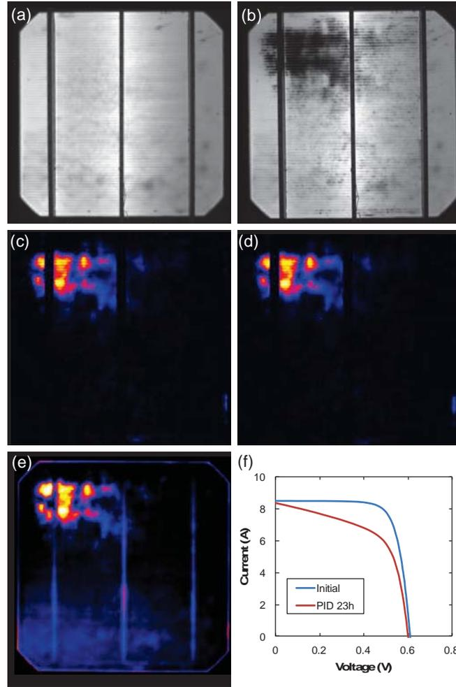
Figure 6.1 Images before and after PID Stressing at 60 °C/0% RH, -600 V, 23 h. (a) EL Image before PID Stressing, (b) EL Image after PID Stressing, (c) DLIT Image under +0.5 V, (d) DLIT Image under -0.5 V (e) ILIT Image (f) I-V curve
