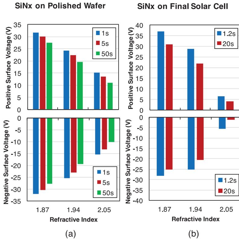
Figure 5.4 Positive and Negative Surface Voltage after Corona Charging on SiN<sub>x</sub> Films with Various Refractive Index. Different Color Bars in a Group of RI Represent Different Times after Corona Charging Cessation. (a) SiN<sub>x</sub> Film on Polished Wafer, (b) SiN<sub>x</sub> film on Finished Solar Cell.
