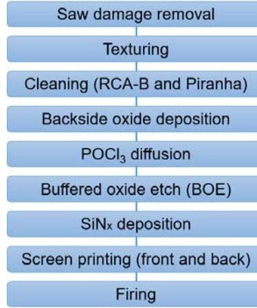
Figure 5.1 SPL Standard Cell Process Flow
