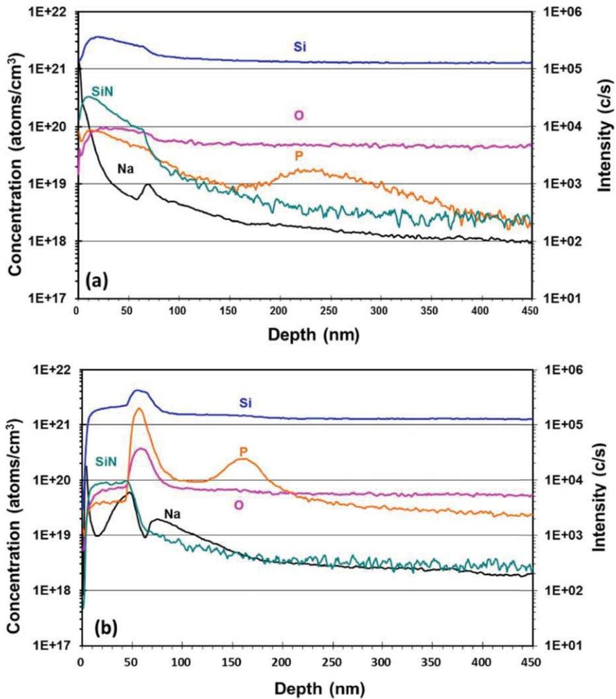
Figure 2.34 SIMS Depth Profile of (a) a Standard Solar Cell and (b) the PSG Layer Added to the Solar Cell [66].
