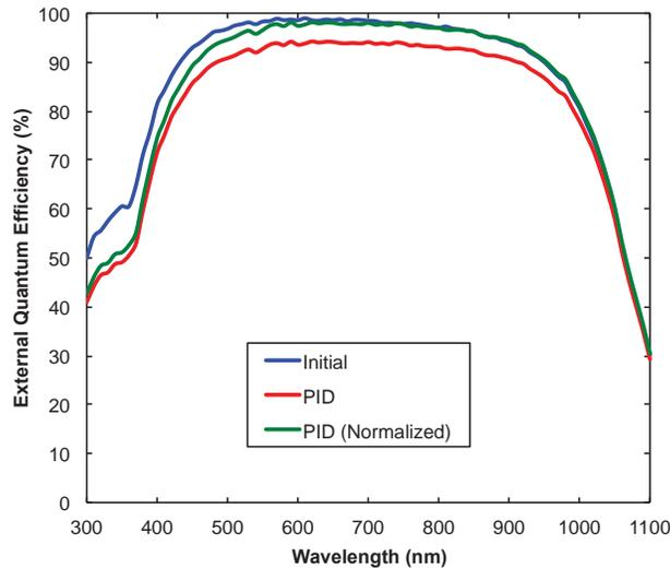
Figure 4.6 QE of Bare Cell (M1; setup 2) before and after PID 80 °C/24 h/-600 V. QE of PID Affected Area Characterized by EL was carried out. QE of PID Stressed Cell is normalized.
