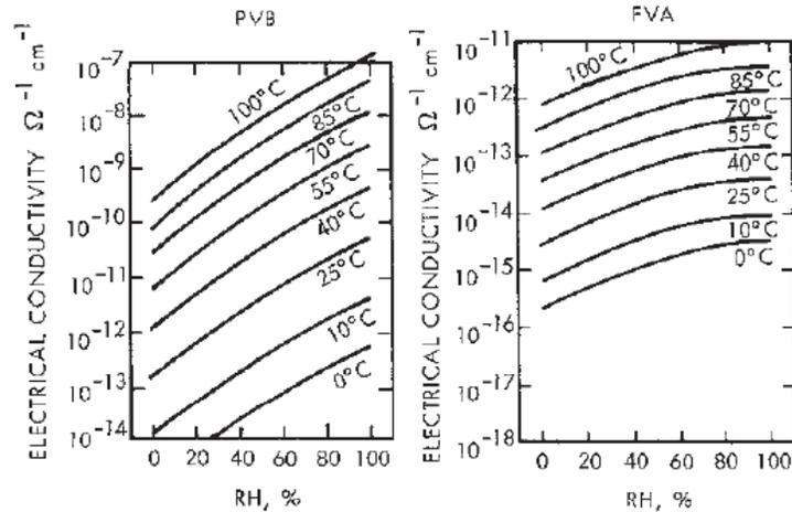
Figure 2.5 Electrical Conductivity of PVB and EVA as Function of Temperature and RH [26].
