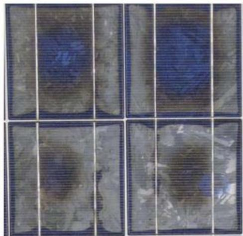
Figure 2.4 Removal of the SiN<sub>x</sub> ARC after 1000 h in 85 °C/85% RH with -600 V [19].
