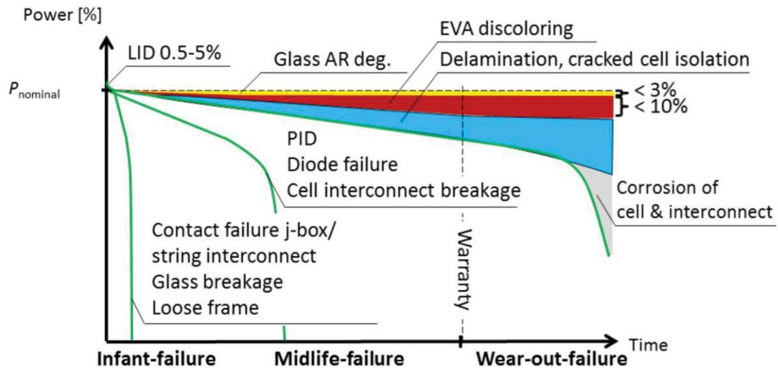
Figure 1.5 Three Typical Failure Scenarios for Wafer-Based Crystalline PV Modules [9]
