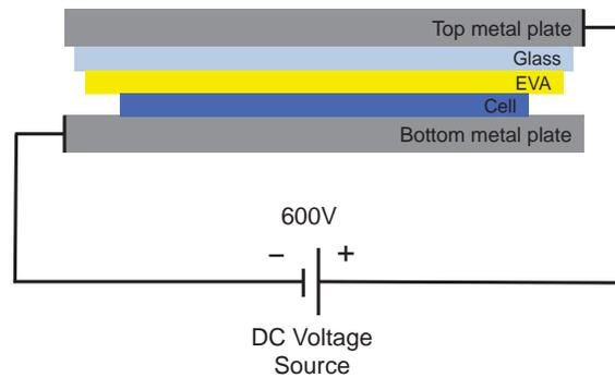
Figure 5.2 PID Test Setup without Module Lamination
