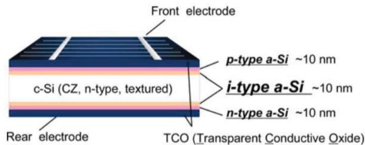
Figure 2.35 HIT Cell Structure [84].
