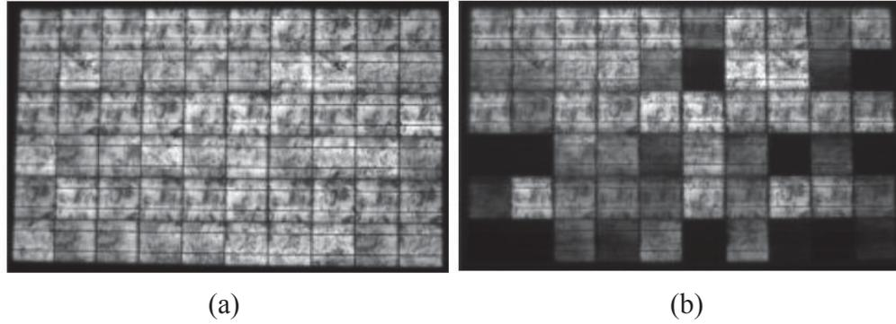
Figure 2.14 EL Image of a Module (a) Before and (b) After PID 100 h,  $-1000$  V [28].
