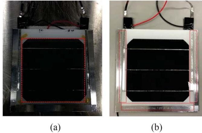
Figure 7.1 Photograph of Two One-Cell Coupons. Red Dotted Areas are the Locations where the Willow Glass (a) Sheet or (b) Strip was placed. (a) coupon A; (b) coupon C.
