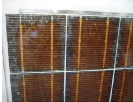
Figure 1.6 Discoloration of the Encapsulant due to UV [12]
