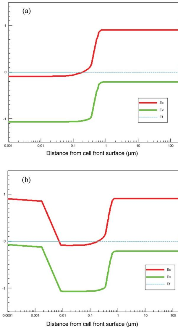
Figure 4.3 Sentaurus Band Diagram for a Solar Cell, (a): No Surface Charge, (b): with Negative Surface Charge ( $-1 \times 10^{15} \text{ cm}^{-2}$ )
