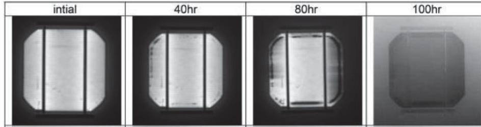
Figure 2.16 EL Image of a Cell during PID Test,  $-1000\text{ V}$ , a Front Glass is Flooded with Water [28]
