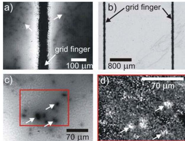
Figure 2.23 (a) Lock-In EBIC Image of the PID-Stressed Cell; (b) Lock-In EBIC Image of the Non-PID-Stressed Cell; (c) Detailed Lock-In EBIC Image of the PID-Stressed Cell; (d) SIMS-Difference Na<sup>+</sup> Map of Red Area in (c) [40]
